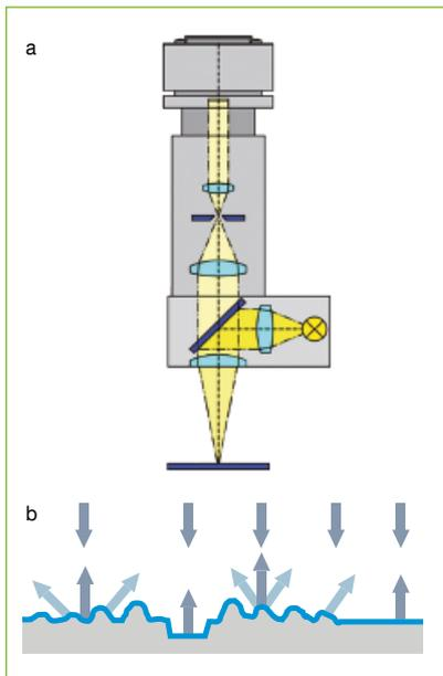
Fig. 4 Scheme of the LASM (a) and optical scheme of bright-field illumination (b): The light directed at the sample is reflected by surfaces parallel to the sensor. Light reflected from structures areas and edges is reflected away from the sensor and appear dark.
