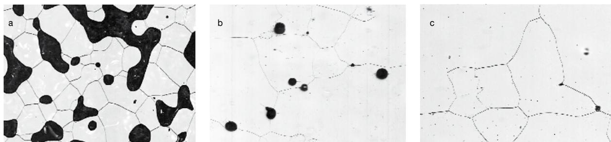
Fig. 3 Ice core sample images from different depths. All scans are obtained using the large area scan microscope. The ice core image from 60 m depth (a) shows grain boundaries and pores. These inclusions become rarer and smaller with depth (b; 615 m depth). Finally, at a depth of 1035 m, almost all gas inclusions have transformed into air hydrates.
