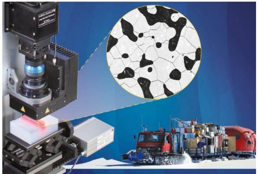
Fig. 1 Large area scan macroscope for the analysis for microstructure of polar ice cores. (Source: Lars Berg Larsen, NEEEM ice core project)
