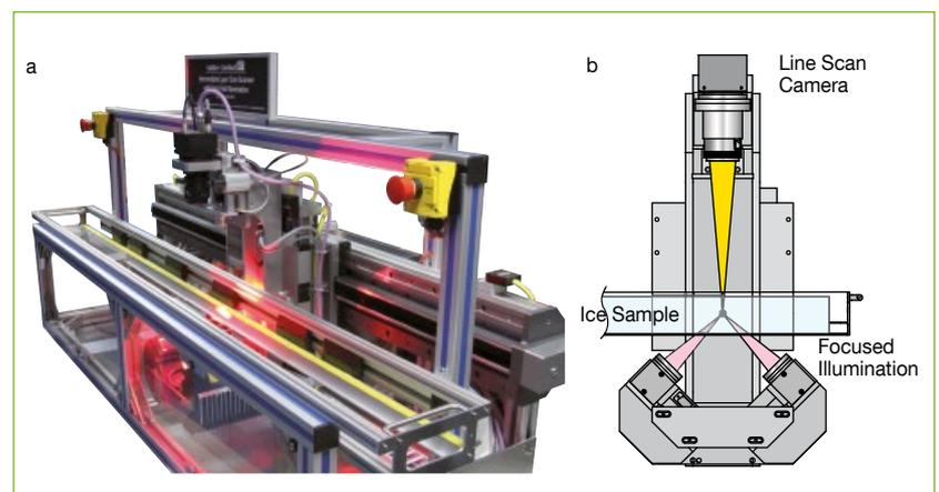
Fig. 5 Intermediate Layer Core Scanner (ILCS, a) and optical scheme (b). The camera located above the ice sample is moved synchronously to an indirect light source that is mounted below the sample. Relevant structures are visualized using the dark-field illumination technique. The light from the two sources is focused into the sample from two sides. Only light scattered in the sample is directed back to the camera, direct light from the illumination unit does not reach the sensor.
