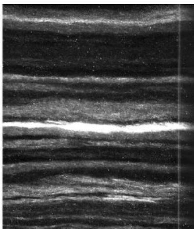
Fig. 6 Stratigraphic scan showing the layered structure of the ice core. Transparent ice appears dark while micro-inclusions like mineral dust or salt particles form brighter visible layers. Colored layers indicate volcanic ash horizons, grey layers mineral dust and salts inclusions.
