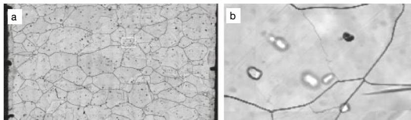
Fig. 2 Image of a  $20 \times 45 \text{ mm}^2$  wide ice core section mapped by an optical microscope. A series of 300 images is necessary for the fully reconstructed picture (a). A single picture,  $2.5 \times 1.8 \text{ mm}^2$  in size, is marked with a white rectangle and shown in (b). The dark lines show grain boundaries, the inclusions are air hydrates. [2]
