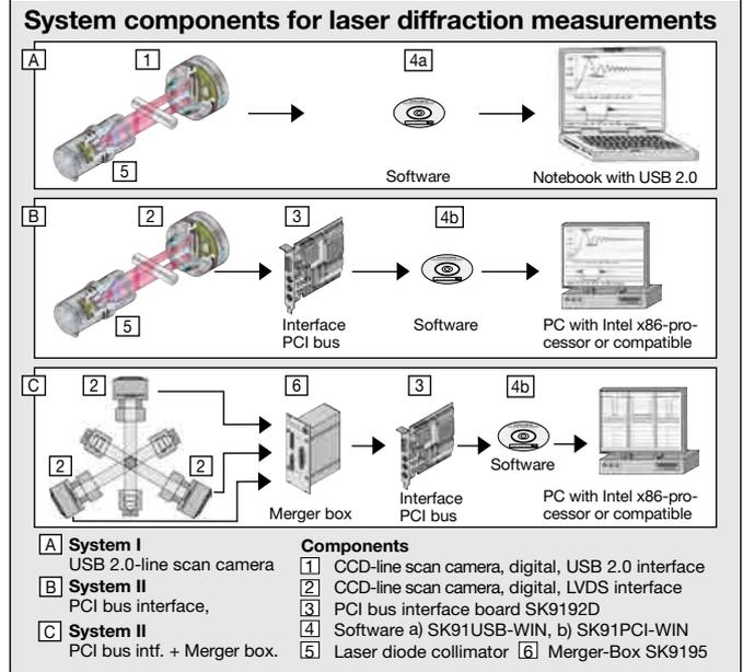
**Fig. 11:** System components of the laser diffraction measuring system
