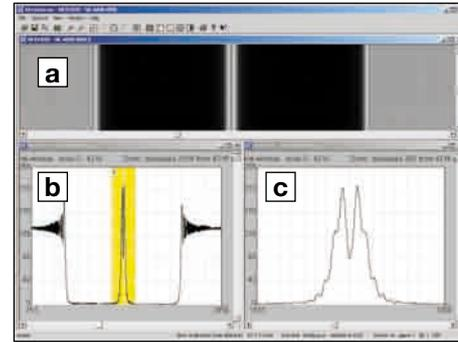
**Fig. 3:** Diffraction by two round rods in a distance of 1mm. (Measurement setup see Fig. 2, Objects 2, 2.1)
