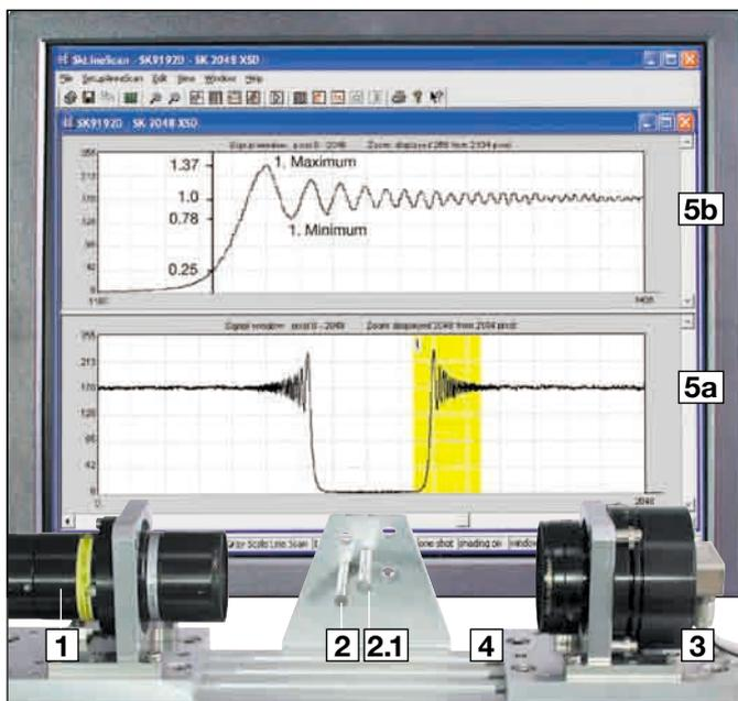
**Fig. 2:** Measuring station laser diffraction
