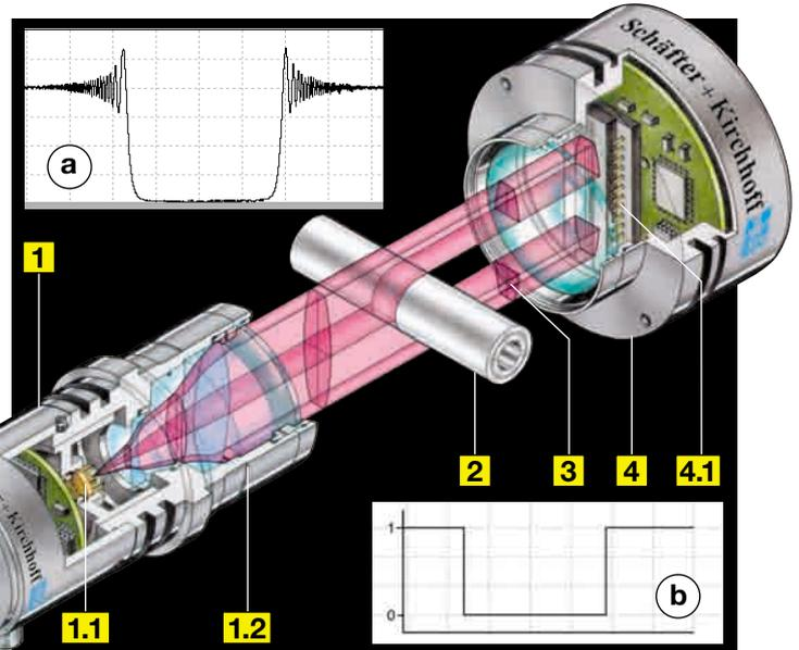
**Fig. 1:** Schematic measurement configuration and beam propagation with laser diffraction. 1. laser diode collimator, 1.1 laser diode, 1.2 lens for collimating the divergent laser diode radiation, 2. object under test, 3. partial obscured laser radiation, 4. CCD-line scan camera, 4.1 CCD-line scan sensor. The collimated beam is elliptical (vertical beam size 32mm).
