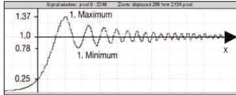
**Fig. 5:** Display of the intensity distribution orthogonal to the diffracting edge.
