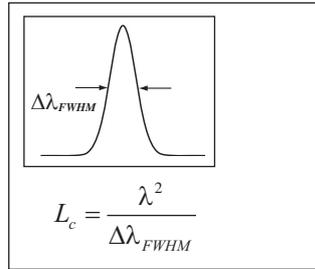
The particular application determines whether a long coherence  $L_c$  (here given for a Gaussian spectrum) or a short coherence is desirable. Non-stabilized singlemode lasers with stochastic changes of the wavelength also exhibit stochastic changes in coherence behavior.
