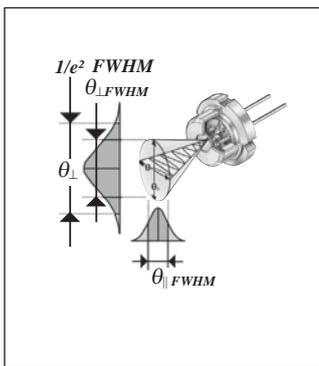
The beam can be characterized by the divergence  $\theta_{\perp} \times \theta_{\parallel}$  measured perpendicular and parallel to the active surface area at the  $1/e^2$ -level (= 13.5%).
