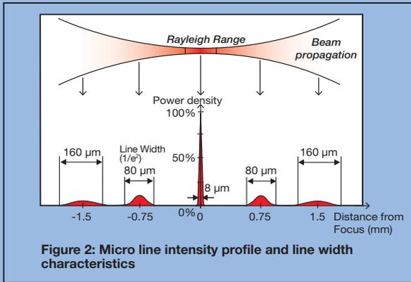
Figure 2: Micro line intensity profile and line width characteristics
