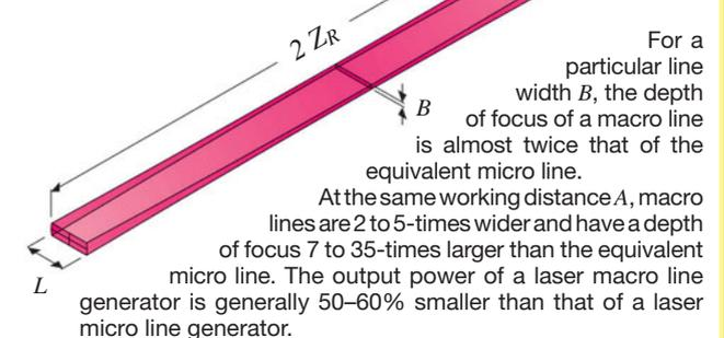
**Laser Macro Focus Generators** generate laser spots with lower power density and an extended depth of focus. The intensity profile is approximately Gaussian. The line width  $B$  is replaced by the spot diameter in the formula to reveal the depth of focus.
