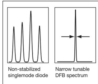
The emitted wavelength can be kept constant in a number of ways. External temperature control is possible using integrated or external Peltier elements and temperature sensors (see 48TE SOT-...). Most laser diodes also have an integrated monitor photodiode, providing feedback for control of the laser power.
