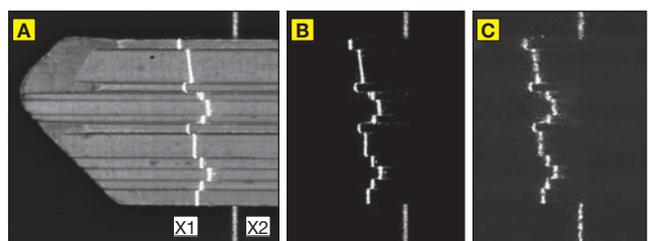
**Figure 1: 3D profiling by use of laser light sectioning**
