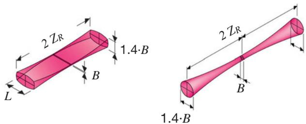
**Laser Micro Focus Generators** produce laser spots with high power density and a Gaussian intensity profile. The line width  $B$  is replaced by the spot diameter in the formula to reveal the Rayleigh range.
