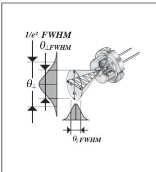
The microscopic cross-section of the laser diode active area of 1 x 3 μm results in emitted radiation that is divergent. Most laser diodes have a cone of divergent radiation with an elliptical cross-section and an approximately Gaussian intensity distribution. The ellipticity can be overcome with the help of anamorphic optics.
