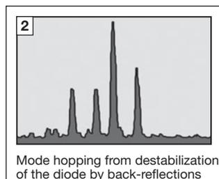
Faraday Isolators (48FI-5-...) can effectively prevent back-reflection into the diode [1].
