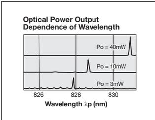
The emitted spectrum is influenced by the diode temperature and diode current, as well as the geometry of the laser cavity. The front face and the end face serve as a Fabry-Perot cavity allowing multiple longitudinal modes.
