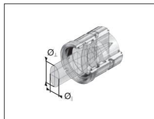
Even a collimated beam exhibits minimal divergence, since the beam diameter varies (for large distances) with the distance  $A$  from the laser diode collimator. The resulting beam divergences of the collimated beam  $\vartheta_{\perp}$  and  $\vartheta_{\parallel}$  depend on the respective beam diameters at the collimator  $\varnothing_{\perp}$  and  $\varnothing_{\parallel}$  and on the wavelength  $\lambda$  of the
