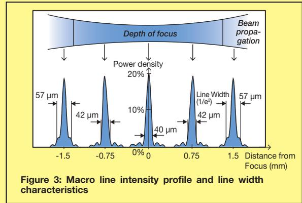
Figure 3: Macro line intensity profile and line width characteristics
