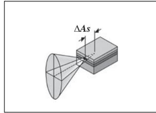
The non-uniform gain profile within the active layer of the laser diode means that some laser diodes show astigmatism. Here, the laser radiation emitted parallel and perpendicular to the active layer does not emerge from one point at the cavity end, but appears to be emerging from two different positions. The distance between these is called the astigmatic difference ΔAs and is between 3–40 μm. Astigmatism can be corrected by using anamorphic optics (5AN-...).
