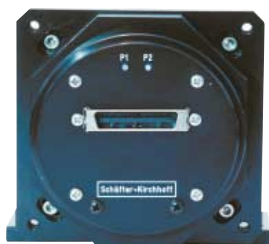
J1 = Mini Centronics 36pin-male, P1 = Gain even, P2 = Gain odd
