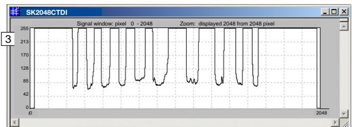
Oscilloscopic displays of CCD line signals (bar code with incident light), SK2048CTDI
