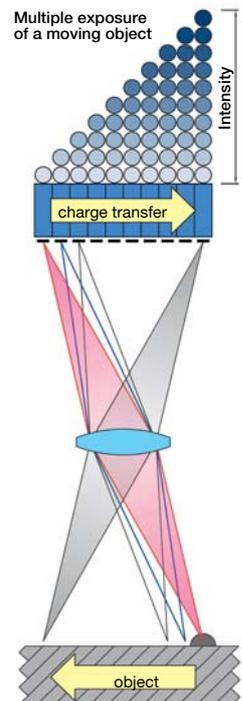
Cameras using Time Delayed Integration (TDI) technology have a sensitivity 96-times greater than conventional line scan cameras. TDI line scan cameras are especially useful for dimly-lit objects (e.g. wafer inspection with dark field illumination) and they can achieve extremely high measurement and scan velocities.
