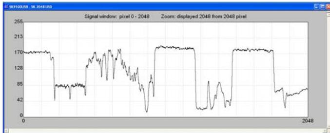
Oscilloscopic display of the line scan camera signal
