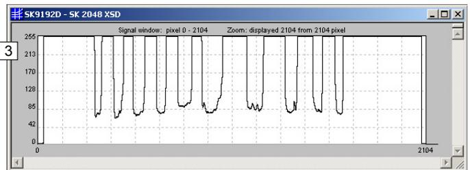
Oscilloscopic signal display of the CCD line scan signal (barcode with incident light), SK 2048 USD
