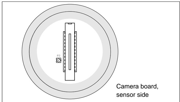
The trimmer P3 is accessed from the front of the camera with the lens taken off.
