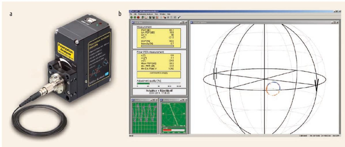
Fig. 5 Polarization Analyzer SK1010A (a) and exemplary PER measurement for an end cap fiber at 488 nm (b). A circle is automatically fitted to the measurement
