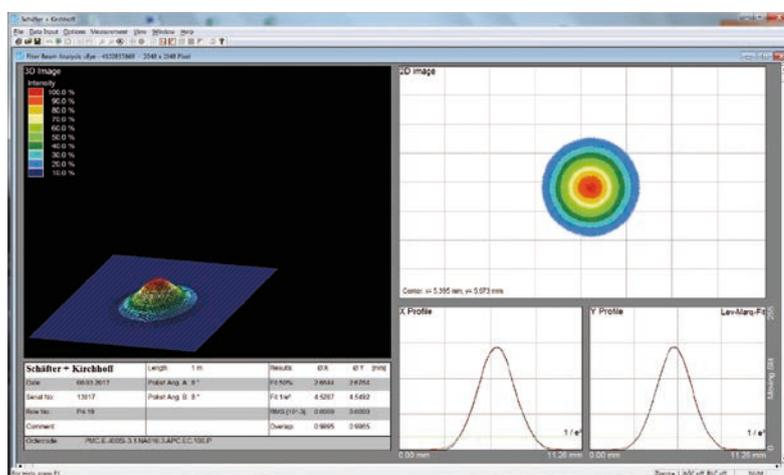
Fig. 4 Exemplary measurement of a beam profile of a fiber with end cap at 488 nm. The  $x/y$  cross section is in very
