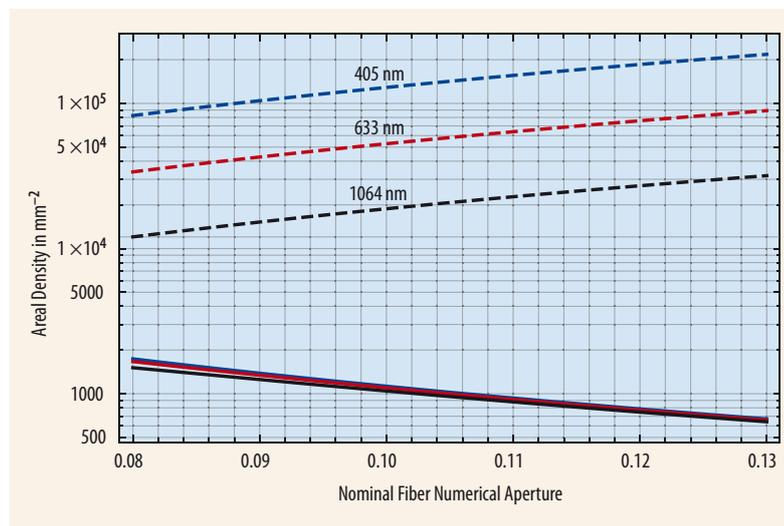
Fig. 2 Areal density at the fiber end-face with (solid lines) and without end-cap (dashed). The areal density is calculated using basic Gaussian beam propagation in a medium. It is much larger without
