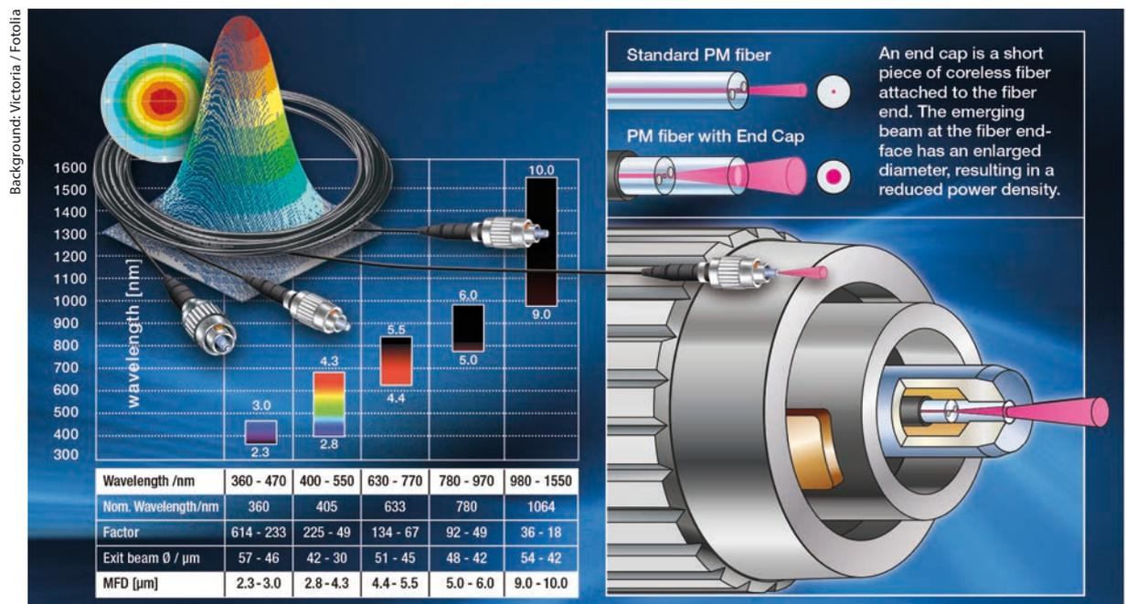
Fig. 1 End caps reduce the power density at the fiber end-face by a wavelength and numerical aperture dependent factor ranging from about 20 to 600. At the
