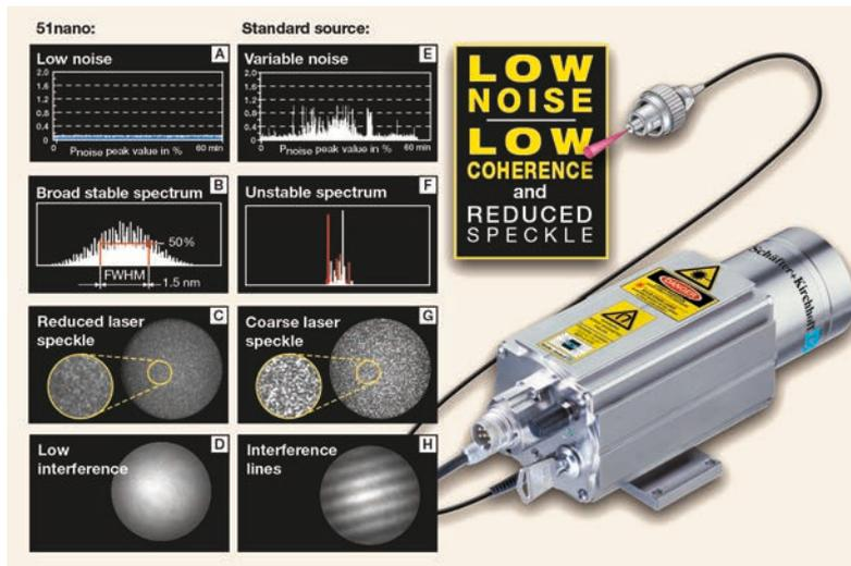
Fig. 3 Laser diode beam source 51nano with reduced coherence length (a–d) compared with a standard laser diode beam source (e–h). Advantages include low noise (<0.1 % RMS, a) because of the
