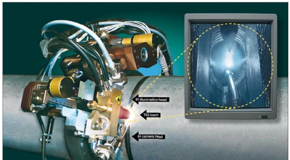
Fig. 1 Arc and laser welding monitor permits remote observation and control of arc and laser welding operations.
