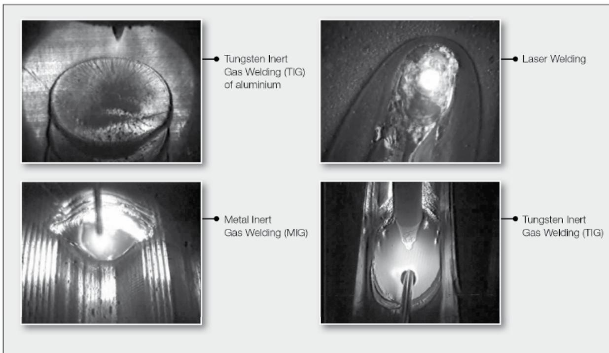
Fig. 2 Still images of different welding processes. For videos see [www.sukhamburg.com/products/arc-welding-monitor.html](http://www.sukhamburg.com/products/arc-welding-monitor.html)
