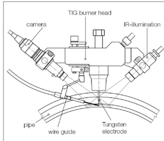
Fig. 3 Optical scheme of a welding monitor.
