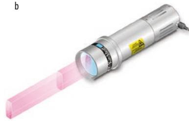
Fig. 4a Measuring the concentric run out of a fan: The collimated laser beam directed onto the line scan camera is tangentially interrupted by the rotating fan, creating a shadow edge in the line signal. The concentricity of the rotation is calculated from the variation of the edge position.
