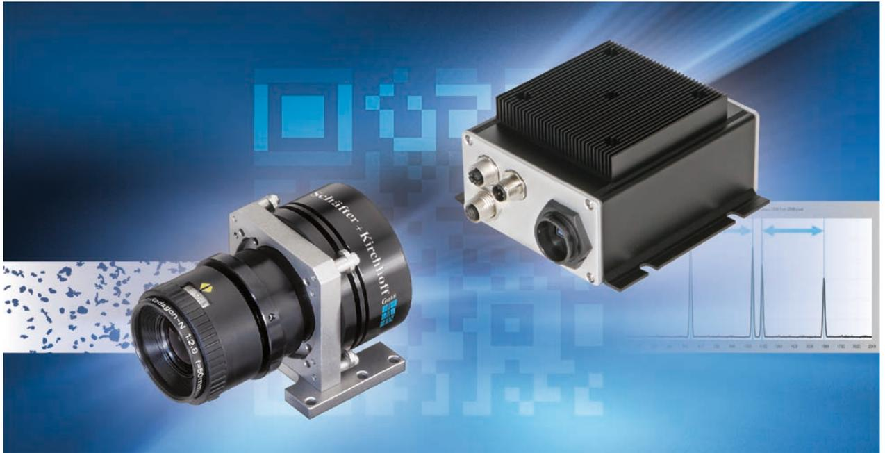
Fig. 1 The Smart Control Box SK91USB3-SC100 is the heart of a smart line scan camera system. Connected to a USB 3.0 line scan camera it provides standalone image acquisition and analysis capabilities to downstream PLC devices or process control computers.
