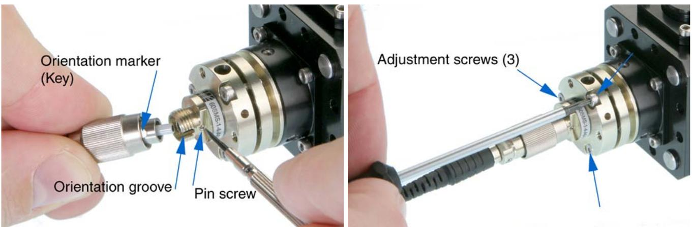
Figure 4: Left. Ensure that the pin screw is loosened before inserting the fiber connector. Right: Coarse tilt adjustment of the laser beam coupler with the three headed screws.
