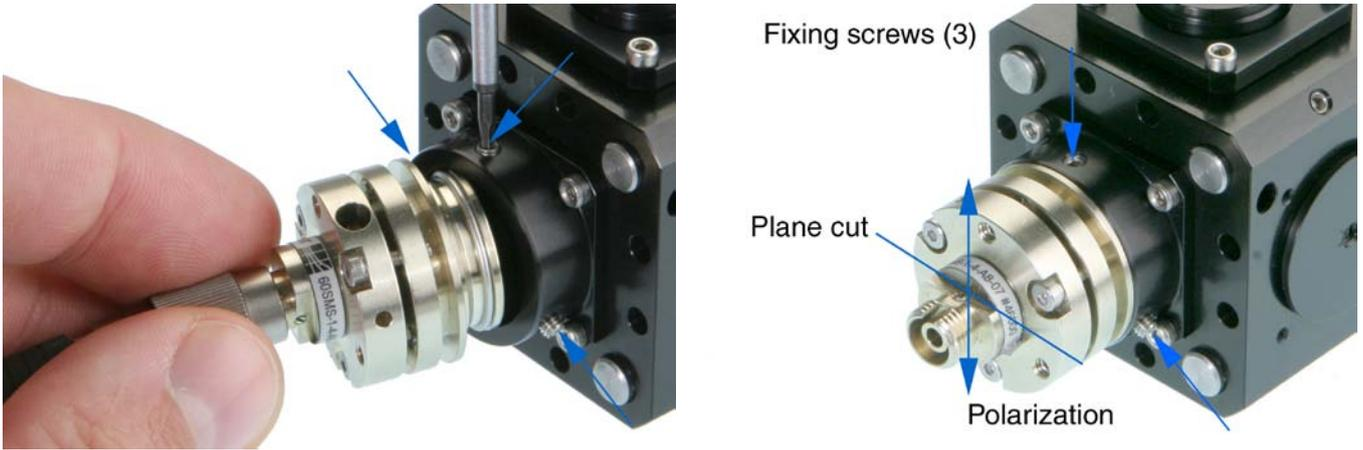
Figure 3: Left. Attach the laser beam coupler to the adapter flange with three radially arranged pin screws. Right. For use with a polarization-maintaining singlemode fiber, the plane cut of the laser beam coupler is aligned perpendicular to the laser polarization.
