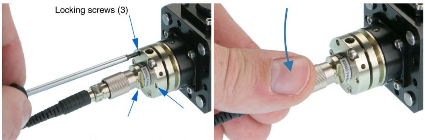
*Figure 5: Left: Fine adjustment and locking of the TILT adjustment by three pin screws. Right: Checking the alignment by pushing the coupler in different directions. If the coupler is aligned correctly, the power emitted by the end of the fiber should always decrease.*
