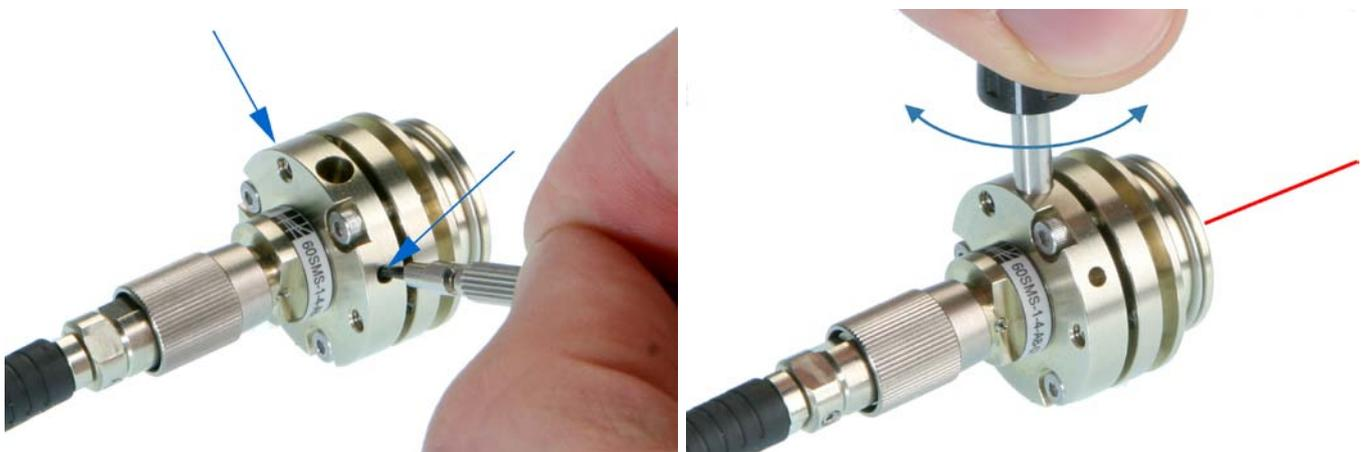
*Figure 6: Left: Loosen the two radially arranged pin screws for loosen the coupling optics. Right: Slightly rotate eccentric key 60EX-5 for collimating the coupling optics.*
