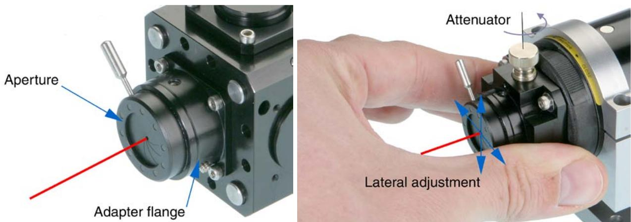
Figure 2: Left: The laser beam and the adapter flange are centered using an aperture. Right: Adapter flange with elongated holes for a lateral adjustment. Completely open the attenuator for the adjustment.
