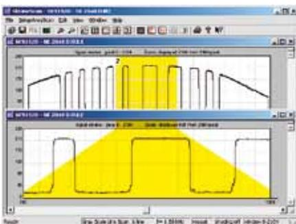
**FIG 3:** The oscilloscopic display of the line scan camera signal produced by the SkLineScan program is ideal for adjusting the camera and lens.
