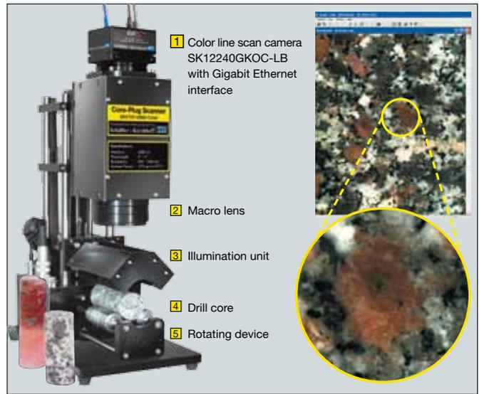
**FIG. 5:** The Drill Core Scanner is a line camera-based mobile imaging system developed for the inspection of geological bore plugs or drill cores. The instrument is highly robust and allows measurements to be performed directly on site.
