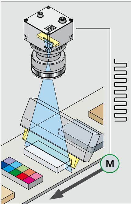
**FIG 1:** The production of a 2D image requires precise synchronization of the line camera sensor and the speed of transport of the object.
