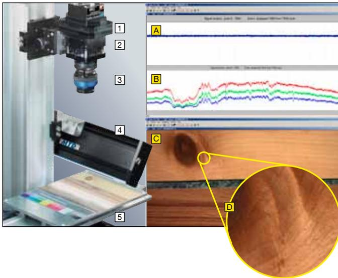
**FIG. 4:** Surface inspection of wood using the SK22800GJRC-XC
