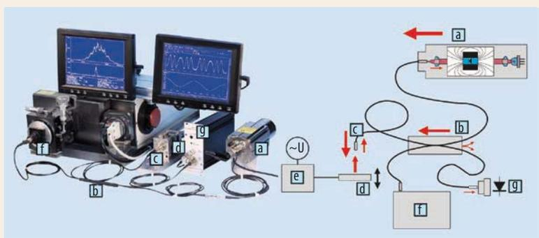
Fig. 4 System components for comparative measurements between a stabilized and a standard laser diode beam source. Light exiting the 51nanoFI (a) is guided through the fiber-optic beam splitter (50/50) (b) onto the mirror (d), which is oscillated by a piezo-element (e). The
