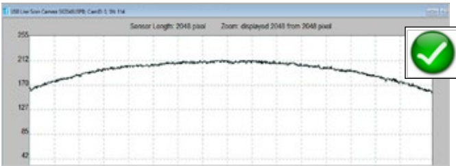
Sensor and line lighting aligned in parallel, symmetric vignetting
