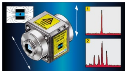
FIGURE 7: Faraday Isolator. Faraday isolators serve as an optical diode. Only light propagating in forward direction is transmitted. Light propagating in the opposite direction is blocked. If back reflections reach the laser source, the once frequency stabilized spectrum (1) is considerably disturbed. Frequency instability (2), increasing noise and a shorter lifetime of the laser beam source are the consequence.
